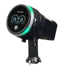
**Upgraded Communications**: The Duo is Genesis Network native, supporting wireless mesh connectivity as well as a wired ethernet option. The Duo can also optionally be connected directly to any plant DCS system via Modbus RTU/ASCII. Using the same memory map as the TCM2, upgrading to Duo will be seamless.
