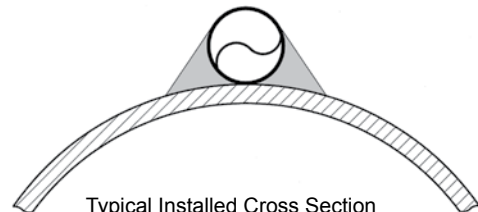
Typical Installed Cross Section (Fillet application)
